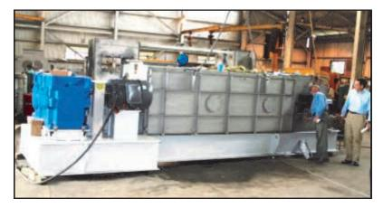
All of Vincent's screw presses can be made vapor tight and ATEX certified. This VP-24 is used in a pectin application.
