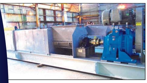
This VP-24 was built for Corn Wet Milling and is equipped with the optional inlet hopper screen.
