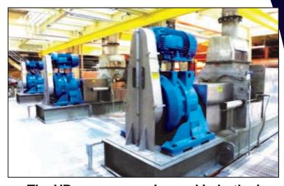
The VP screw press is used in both virgin and recycle mills to press waste streams and screen rejects.
