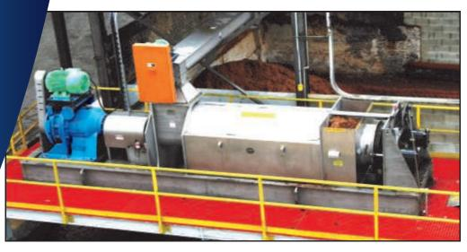
The VP-24 screw presses are used in dewatering tobaccostems and dust.
